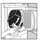
The filter in the inner door must be removed for cleaning.
