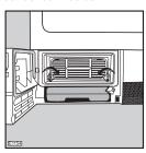
To pull out the condenser, first turn the two red stops downwards and then remove the condenser unit holding it at the handle.
