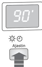
**Before you start the programme**, if you wish to delay the start, press the Delay Start button repeatedly, to select the desired delay. The relevant light will illuminate.
