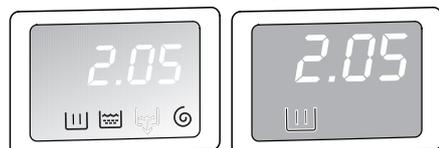
After the machine has started, only the running icon stays on. When the programme has finished, a flashing zero (**0.00**) is displayed.
