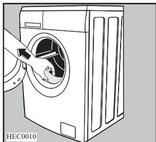
7. Fill the smaller upper hole and the two large ones with the corresponding plastic plug caps supplied in the bag containing the instruction booklet.
