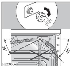
3. Set the hose correctly by loosening the ring nut.
