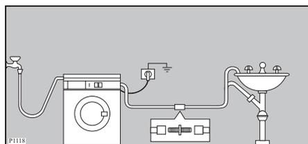
The drain hose may be extended to a maximum of 4 metres. An additional drain hose and joining piece is available from your local Service Centre.
