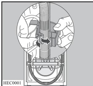
3. With a suitable spanner unscrew and remove the central rear bolt **A**. Slide out the relevant plastic spacer.
